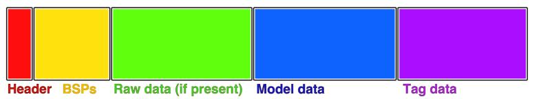
This is a diagram of the cache file structure in the order output by tool.exe. All cache files start with a map header. This header is exactly 2048 bytes in length.
